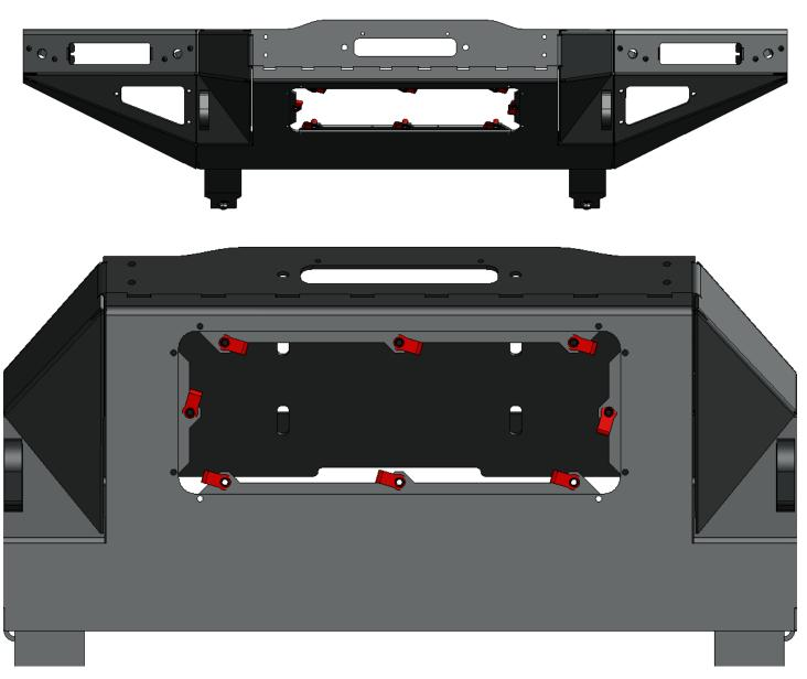
b. Use 8 of the included M8 button head bolts to secure the center filler panel to the center section of the RCI Bronco bumper.
