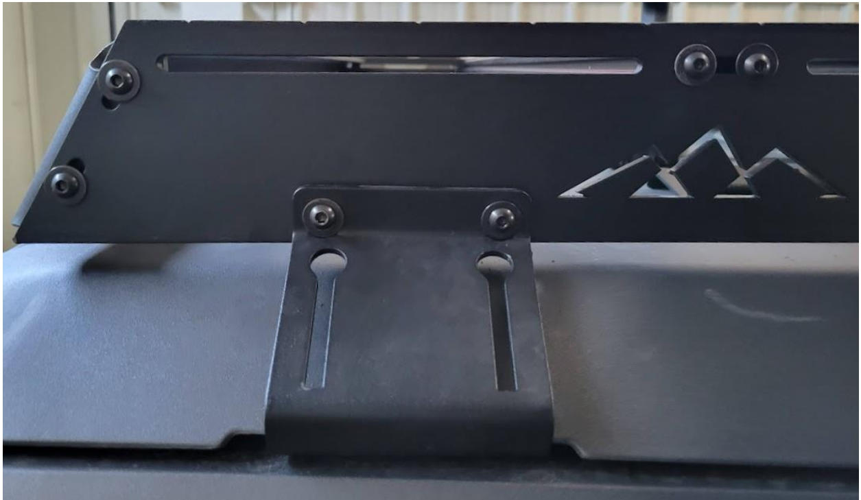
Figure 11. Installation of outer mount; outer mount installed
