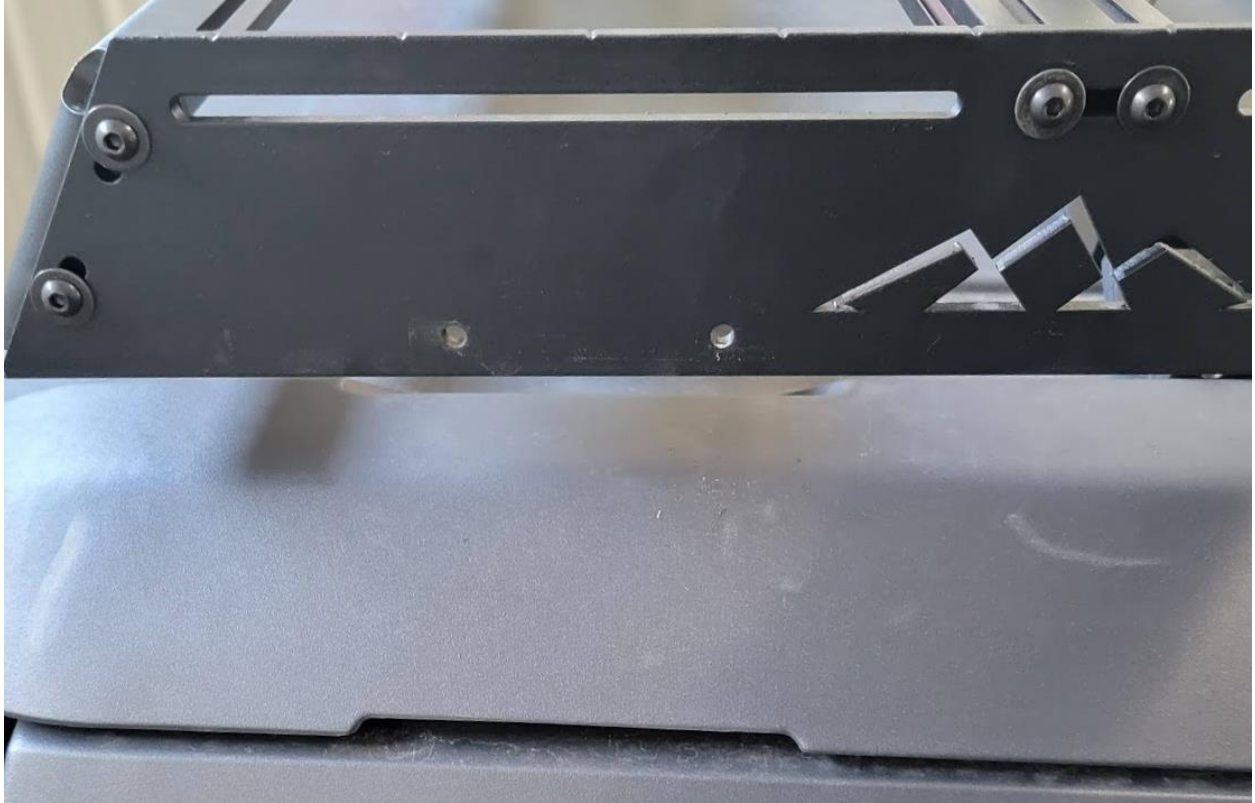
Figure 10. Installation of outer mount; vehicle roof slot
