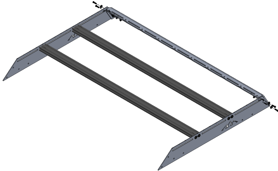
Figure 4. Assembly of half rack subassembly; rear fairing
