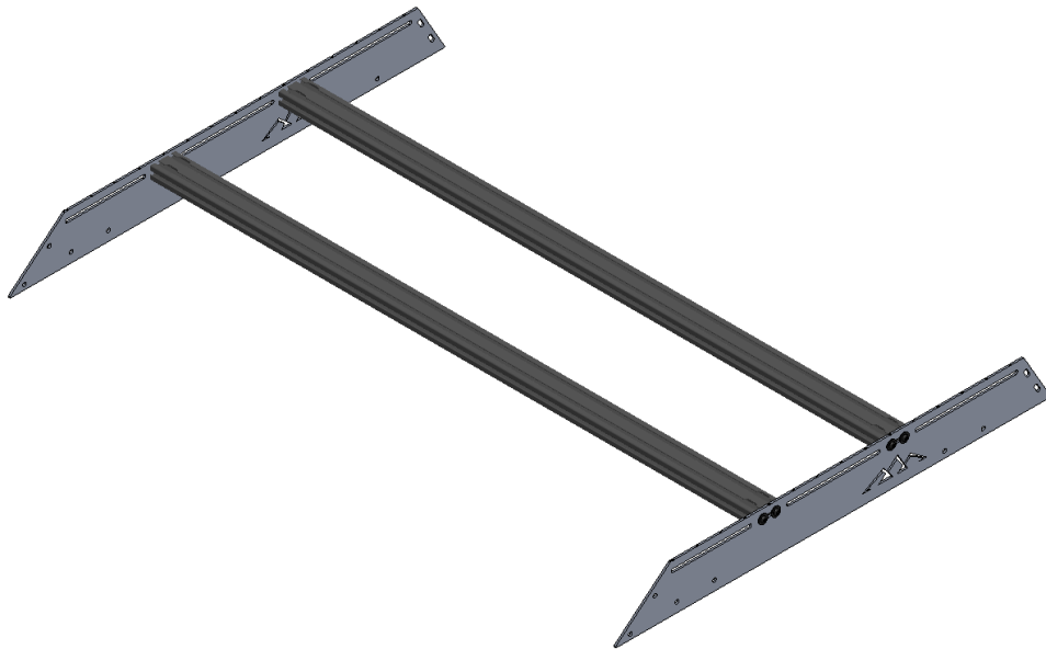
Figure 3. Assembly of half rack subassembly; passenger side panel
