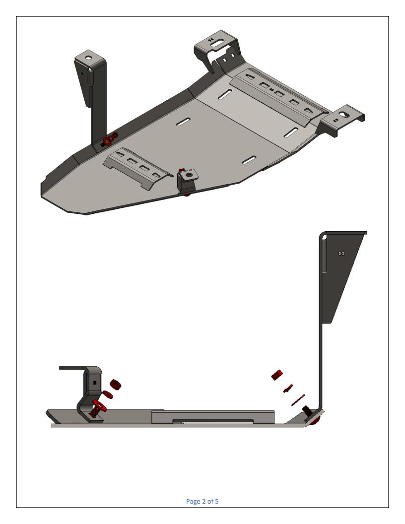
2) Secure the two halves of the skid plate together with the use of four(4) sets of 3/8" Carriage Bolts, Washers, Split Washers, and Hex Nuts.
