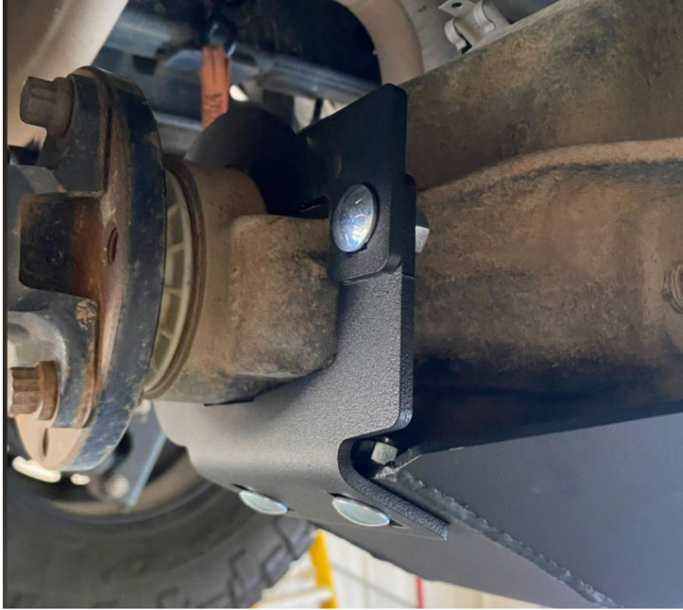
Figure 6: Pinion Clamp Installation
