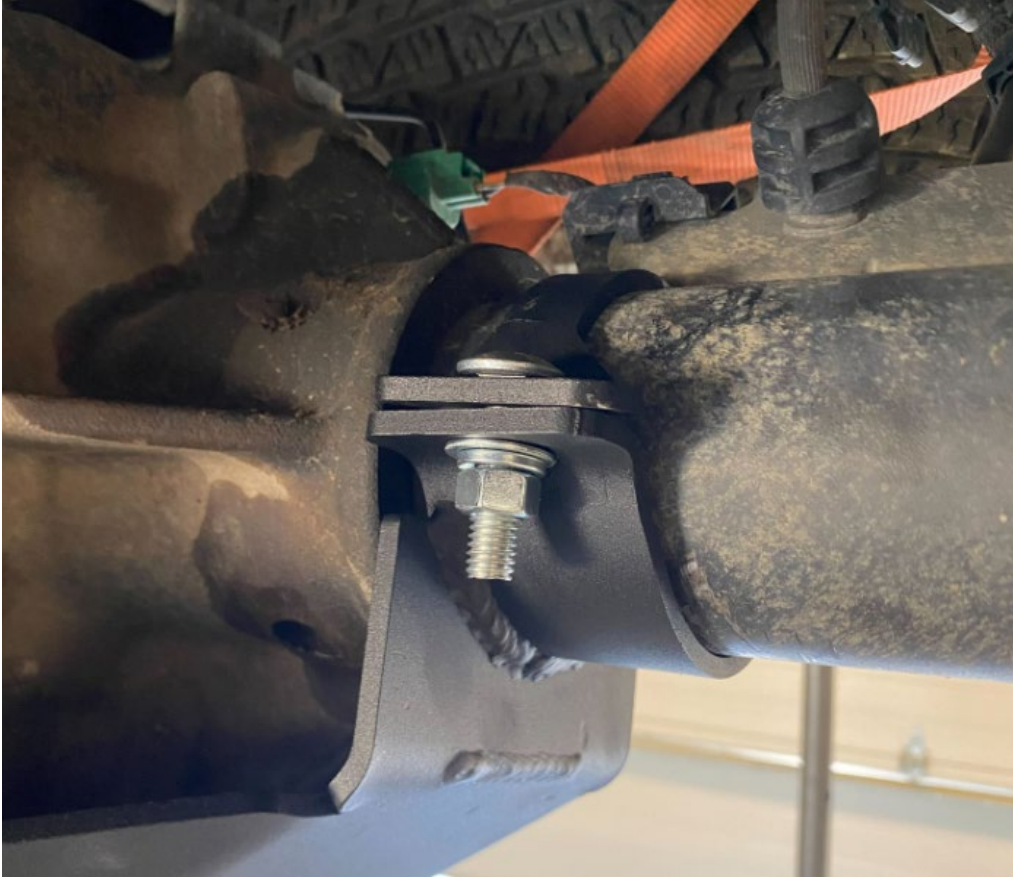
Figure 8: Axle Clamp Installation
