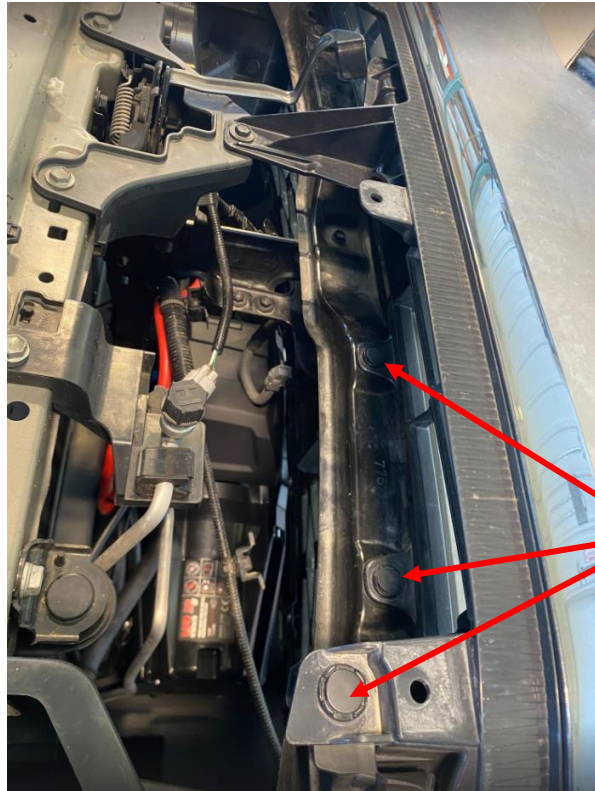
Figure 3: Clips securing grill to crossmember.
