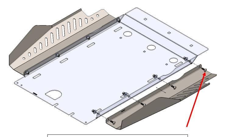
For installation on a EcoDiesel equipped vehicle, do not install the rearmost hardware on either the passenger or driver sides. This will be covered in the transmission skid plate installation guide.
