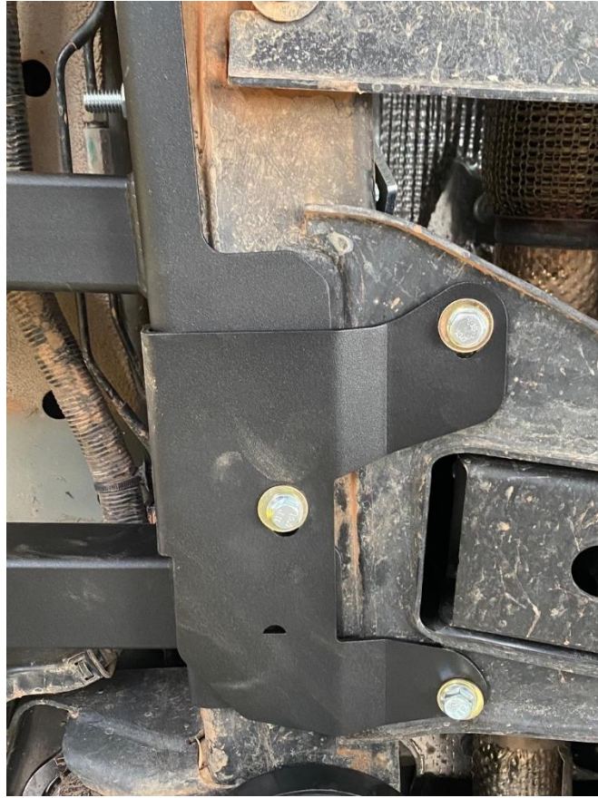
Figure 12 Correct Installation of Mounting Bracket
