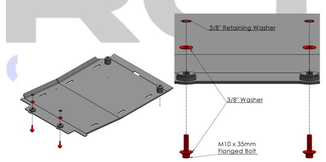
3) Align the front of the Transmission skid plate with the front vehicle crossmember. Thread the bolts into the crossmember until secure but do not tighten; the skid plate will need to be able to move slightly to achieve proper alignment with the rear crossmember.
