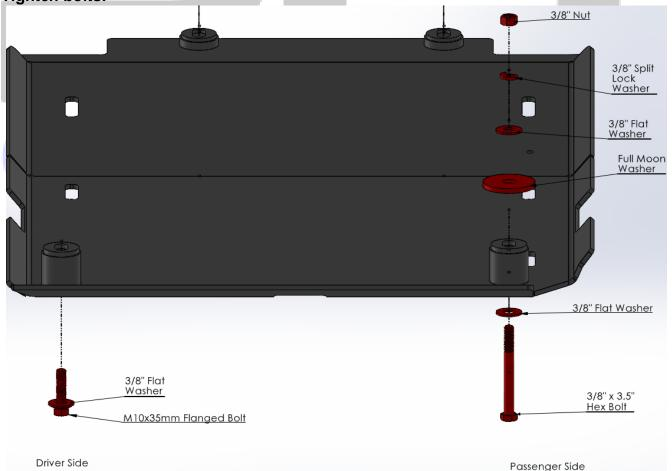
a. If installing the RCI Bronco Transmission skid with an RCI Bronco Engine and Secondary skid plate, please loosely mount the Bronco Engine and Secondary
