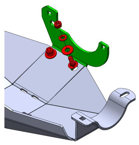
2. Lift the Rear Differential Skid assembly up to the rear axle of the vehicle as shown
