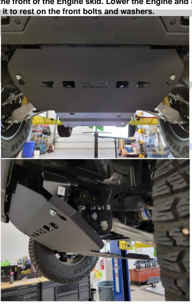
6) Lift the rear of the Secondary skid package until it contacts the vehicle chassis. Loosely install a set of 3/8" washers(2) and M10x35mm bolts(2) in the rear-most mounting points of the Secondary skid.
