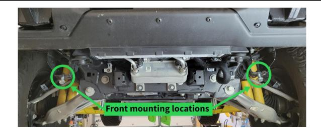
5) Lift the assembled Engine and Secondary skid package to their approximate final location. Pass the washer and bolt assembly installed in step 4 through the keyhole shaped cutouts at the front of the Engine skid. Lower the Engine and Secondary skid
