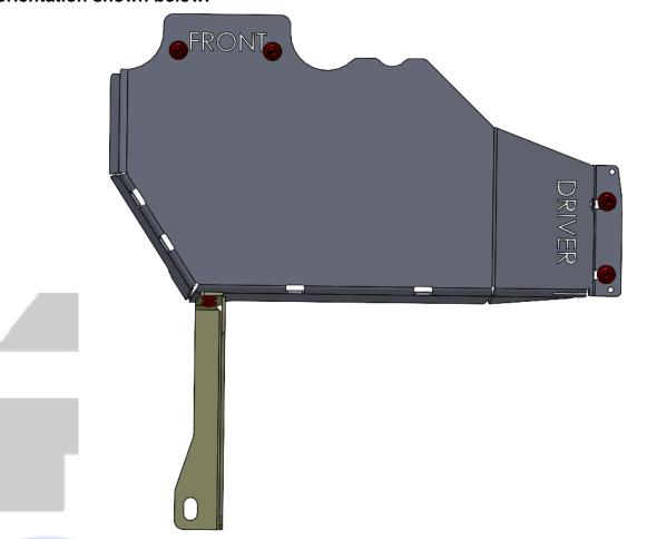
6) Adjust the Transfer Case skid plate to align with the mounting locations present on the central factory crossmember.
