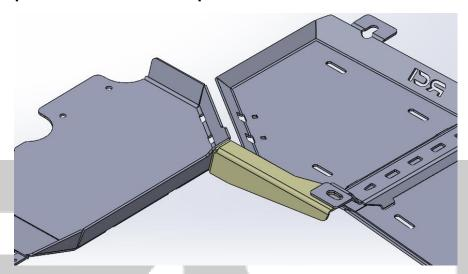
b. If installing the RCI Bronco Transfer Case Skid Plate in conjunction with the RCI Bronco Frame-Mounted Rock Sliders, install the Mounting Bracket "Above" the fuel tank strap or fuel tank skid/bash plate mount as shown below
