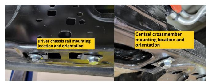
3) Install a set of 3/8" washers(2) and M10x35mm bolts(2) in the speed clip locations on the driver side chassis rail. Leave approximately 1/2" of exposed thread between the bottom of the chassis rail and the washer.
