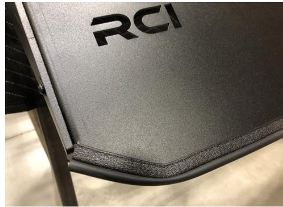
Figure 9: Front fairing weather strip install
