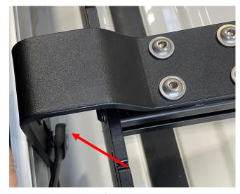
Figure 4: Installing the bracket and awning onto the cross bar
