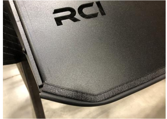
Figure 9: Front fairing weather strip install
