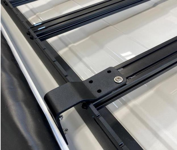
Figure 4: Installing the bracket and awning onto the cross bar
