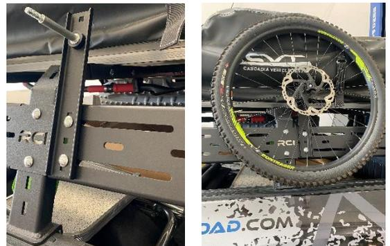
5. To deploy the RTT the tire will need to be removed. The mount will need to be rotated 90 degrees. Loosen the lower threaded knob, remove the bolt directly above the loosened one then rotate the assembly 90 degrees, re-install the short 3/8 bolt and knob.
