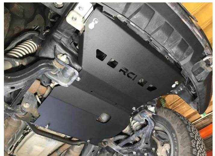
7. Install front skid plate panel first by hanging the skid plate on the bolts installed in step 6. Install bolts with washers at rear of front panel, leaving loose enough for secondary plate to slide in.
