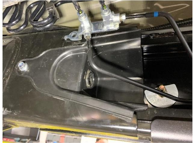
6. Locate the 5 locations on either side of frame with large rectangular or round cutouts. Install each 7/16" bolt with washer, then install backer plates and locknuts on the **inside** of frame rail. For the front two bolts you will have to reach into the frame with an open-end wrench and tighten the bolt from the outside of the frame. Bolts can be installed either with the heads on the outside of frame or on inside depending on preference.
