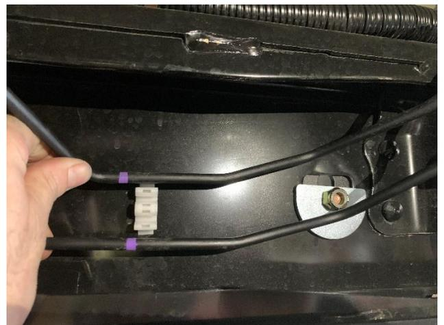
9. For best results, you may choose to drill the additional holes located on the bottom of the frame support flange of each slider. Utilizing these mounting points will increase the strength of the slider for heavy duty use, and minimize flex when lifting truck by the sliders, though it is not required for using the sliders as a jacking point.
